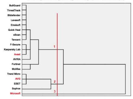
This dendrogram shows the results of the cluster analysis<sup>4</sup>. It indicates at what level of similarity the clusters are joined. The red drafted line defines the level of similarity. Each intersection indicates a group.
