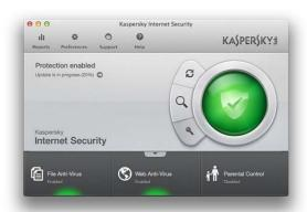
If either of the two main malware protection components is disabled, clicking on the status button opens a dialog box from which the component can easily be reactivated:
